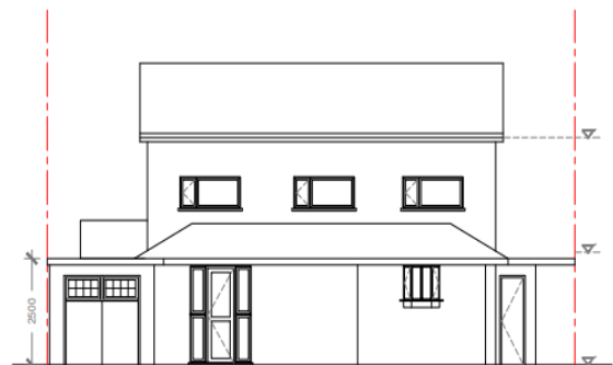
Proposed South Elevation (Front no change) Scale 1:100
