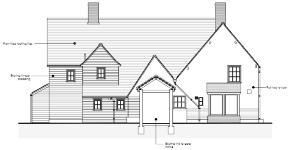
Existing South-West (Rear elevation) Scale 1:50
