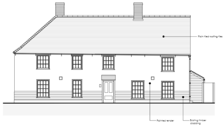
Existing North-East Elevation (Front Elevation)
