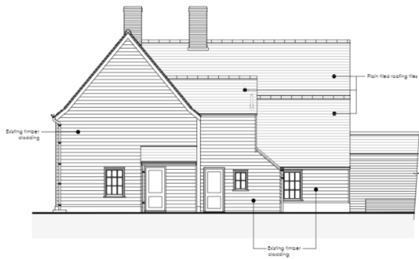
Existing North-West Elevation (Side Elevation)
